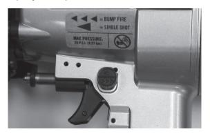
TO PREVENT UNINTENTIONAL TOOL OPERATION AND POSSIBLE INJURY TO YOURSELF OR ANYONE IN THE WORKING AREA, BE SURE TO RELEASE THE TRIGGER AS SOON AS YOU HAVE FINISHED DRIVING FASTENERS.
